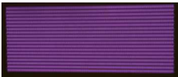
Fig. 1 DCSBD discharge unit producing homogeneous plasma.
