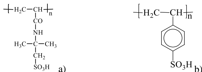
Fig. 1 The structures of the monomer unit PAMPSA (a) and PSSA (b).
