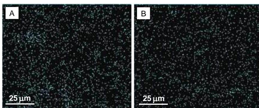
**Fig. 3** Distribution of silver nanoparticles ( $\text{Ag}_2\text{O}$ ) on the surfaces before (A), and after (B) filtration for membrane modified by diffusion method
