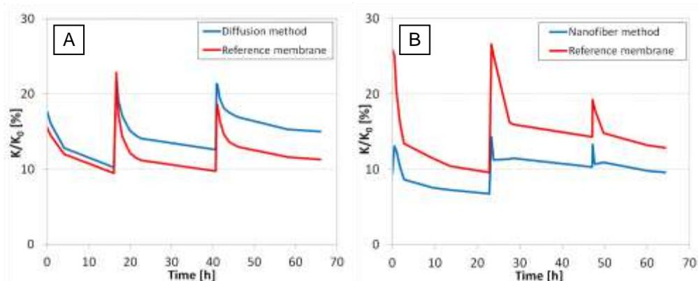
**Fig. 2** Permeability difference (in %) of modified membranes ( $K$ ) compared to original membrane ( $K_0$ ) in the test with activated sludge addition (approx.  $250 \text{ mg}\cdot\text{L}^{-1}$  of suspended solids in the feed)
