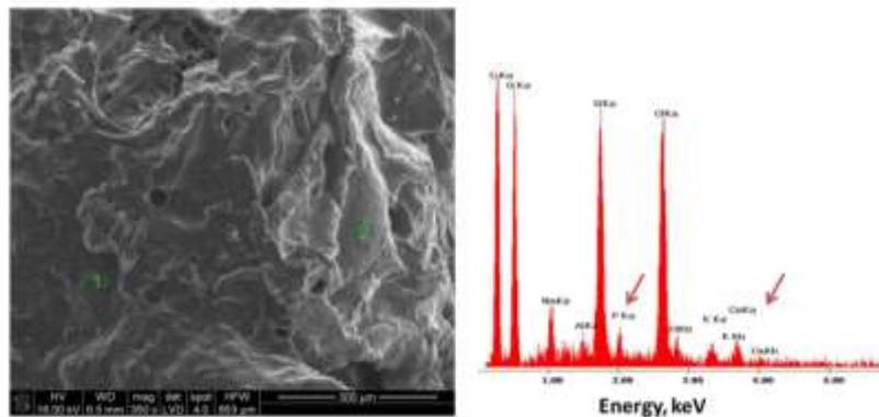
**Fig. 6.** SEM/EDS analysis of a nanocomposite porous scaffold CS/MMT after a bioactivity test
