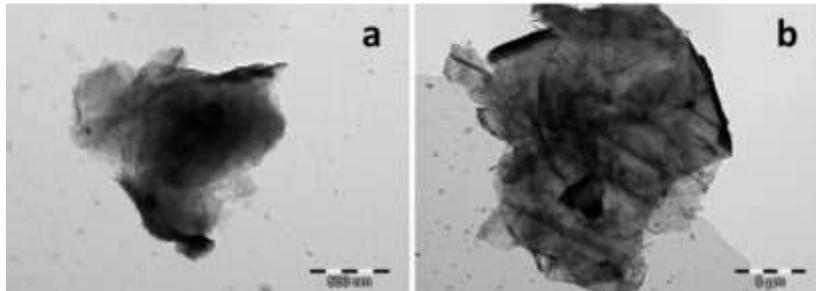
**Fig. 1** Morphology of flake-shaped nanofillers: MMT (a) and GO (b)
