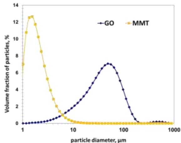
**Fig. 2** Size of nanofillers used in the experiment: MMT and GO (in  $\text{H}_2\text{O}$ ) estimated using the DLS technique
