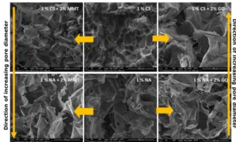
**Fig. 3.** Influence of nanofillers GO and MMT on the microstructure of scaffold samples: NA/MMT, NA/GO and CS/MMT, CS/GO
