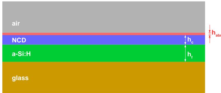
**Fig. 1** Structure of NCD/a-Si:H/glass optical waveguide with adsorbate layer (red colour).
