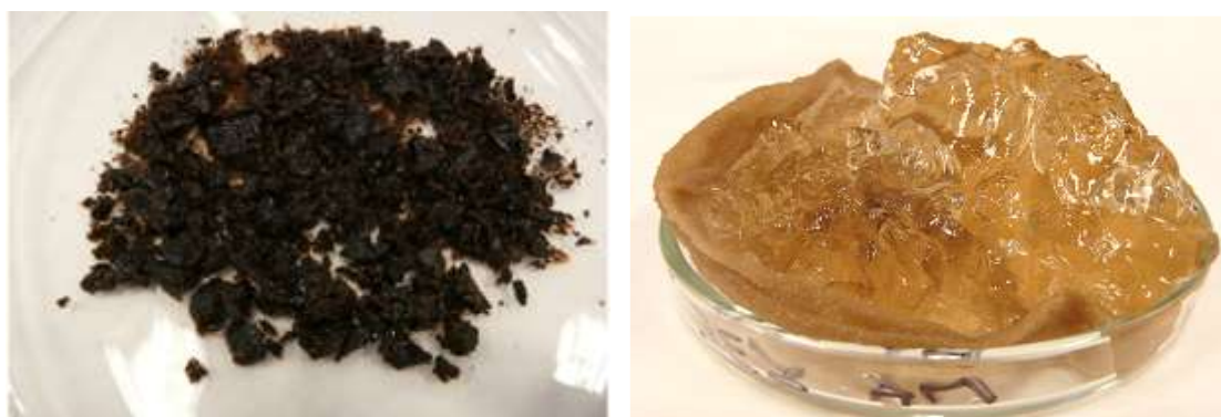
Figure 1 a) Xerogel of superabsorbent polymer. b) Swollen superabsorbent polymer.
