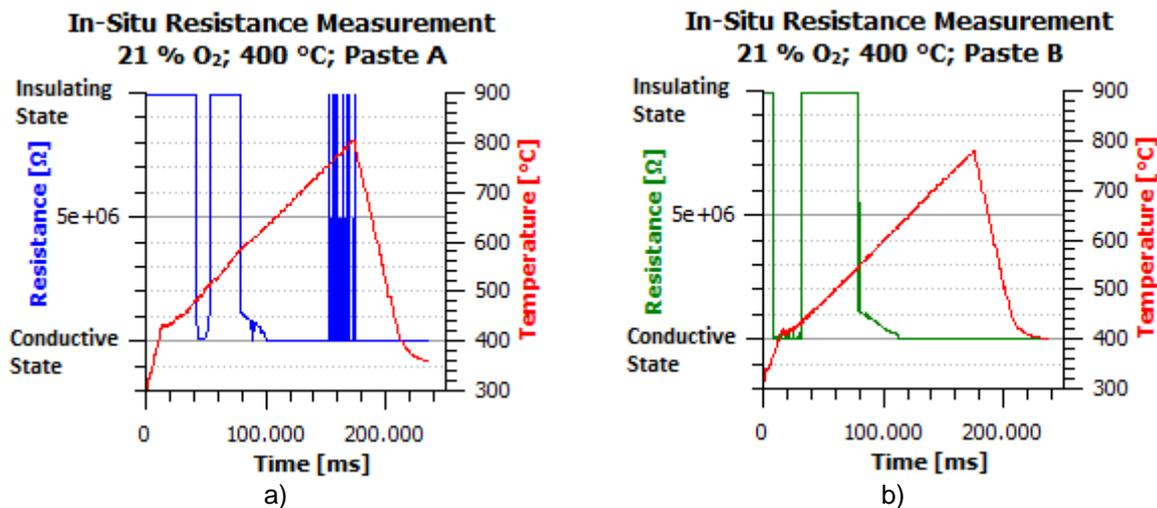
Fig. 5 The dependence of resistance on the temperature using Profile 400.
