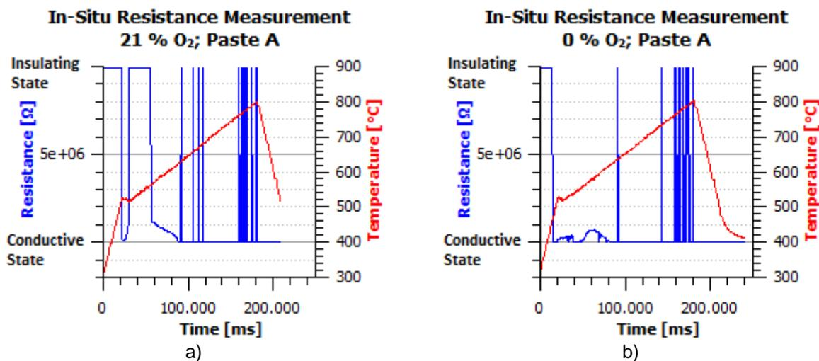
**Fig. 3** The dependence of resistance on the temperature and the content of  $O_2$  for the paste A.
