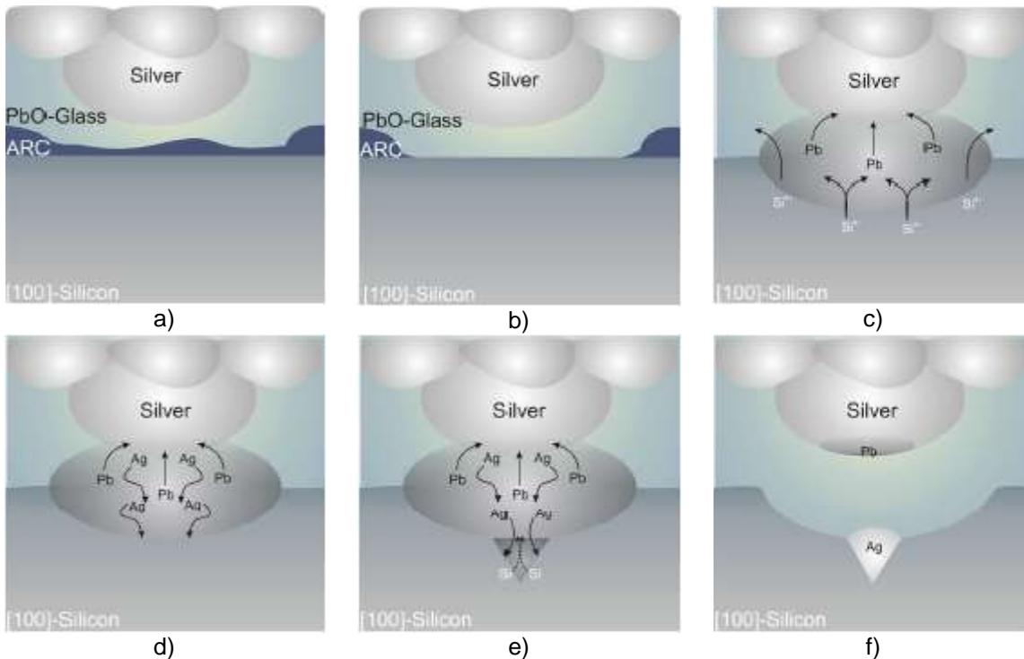
**Fig. 1** Simplified model of contact formation: a) schematic cross section of Ag thick film paste on [100] Si after combustion of organics; b) glass etches through  $\text{SiN}_x$  layer; c) redox reaction between Si and glass, lead (Pb) is formed; d) liquid Pb starts to melt Ag; e) Ag - Pb melt reacts with Si, inverted pyramids are formed; f) on cooling down Ag recrystallises on (111)-Si planes [5].
