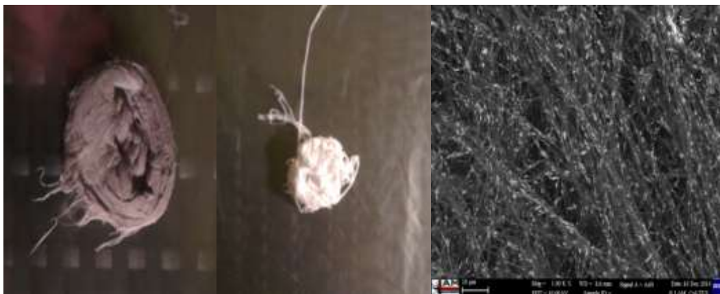
Fig. 3 A) Photo of nanofibers 1:1 CoFe 2 O 4 :PVB, B) clear PVB, C) SEM image of nanofibers 1:2 Fe 3 O 4 :PVB
