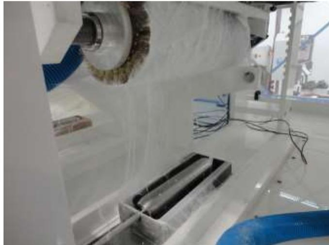
**Fig. 2** View of the machine during the electrospinning process with the bath and brush used as a collector
