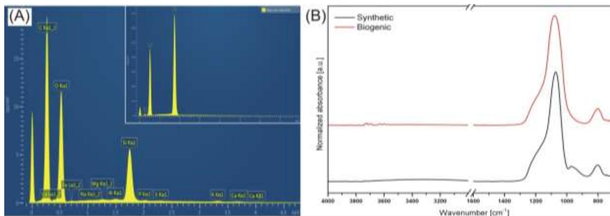
**Fig. 3** EDX analysis of rice husks before and after (inset) the process of chemical pre-treatment **(A)**, FT-IR spectroscopy analysis – a comparison between isolated biogenic and synthetic silicon dioxide nanoparticles **(B)**
