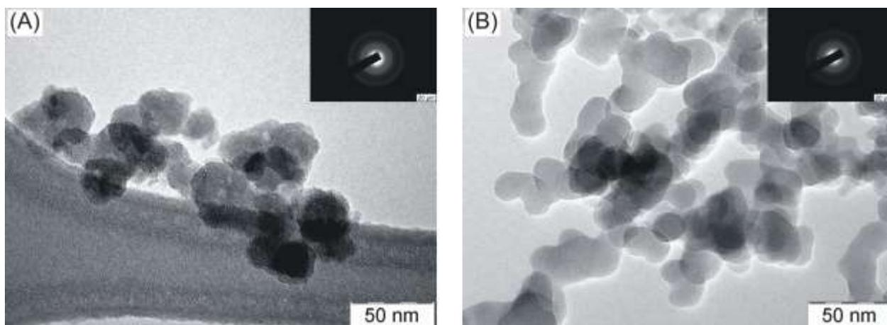
**Fig. 2** TEM images of the biogenic silicon dioxide nanoparticles isolated from rice husks **(A)**, synthetic silicon dioxide nanoparticles type Cab-O-Sil LM-150 **(B)**. Selected Area Electron Diffraction (SAED) showing a diffraction ring – inset
